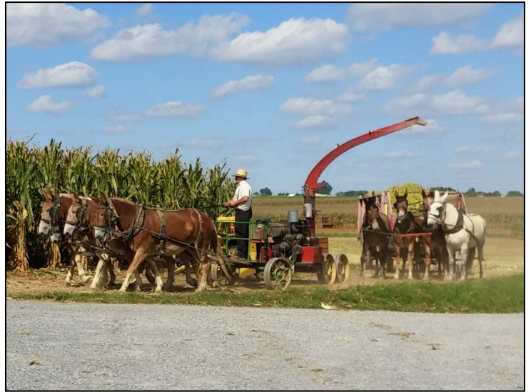
Horse-drawn rig with generator & metal tires
